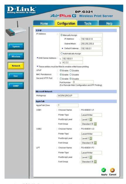
When you select **TCP/IP Protocol** at the **Network** window, the screen below appears. (We recommend that you keep the default settings as shown.) If you need to make changes, make sure to click **Apply** after you have made the changes. (You may wish to make a note of the IP Address.)
